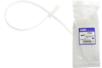
*7" Mounting Hole Cable Tie, 50lb Tensile Strength, Natural, Nylon 6/6, Plenum Rated, Temp Rating -40 to 185 F, Flammability Rating: UL 94-V2, UL 62275 Type*
