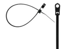
14" Natural Mounting Ties, Bundle Diameter 3/16 to 4, Tensile Strength 120 lbs.
